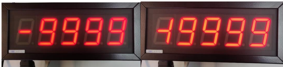
Fig. 14: On the left, minimum value in "FULL DIGIT", -9999. On the right, minimum value in "HALF DIGIT", -19999.
