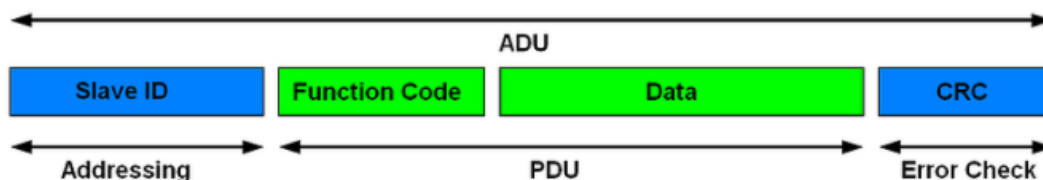
Fig. 26: Modbus/TCP and Modbus/RTU differences.
