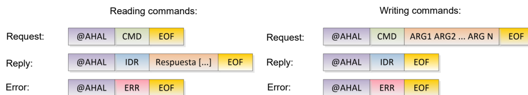
Fig. 4.10 Command Structure for Serial Interfaces
