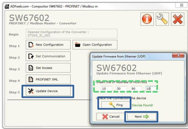
The factory IP address is 10.30.90.10. We must insert this address in the data field to update the device. The “**Ping**” button detects the device before starting the update. If the device is found, the message “**Device Found!**” will appear, press the button “**Next**” and “**Execute Update Firmware**” to continue with the update process. Once finished the process the display will be ready to install with the TIA Portal utility or similar.
