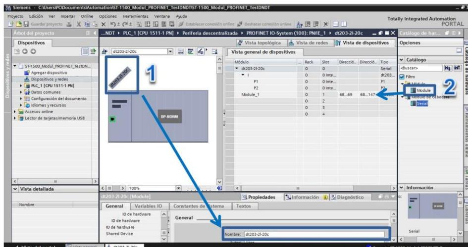
Fig. 10 Assign the E/S addresses of the devices.
