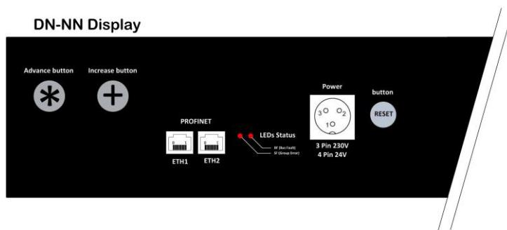
Fig. 2 Connectors and push buttons
