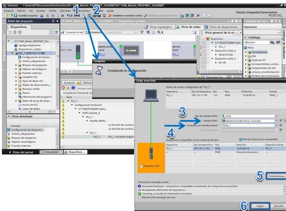
**Fig. 11 Compilation and configuration upload in the PLC**
