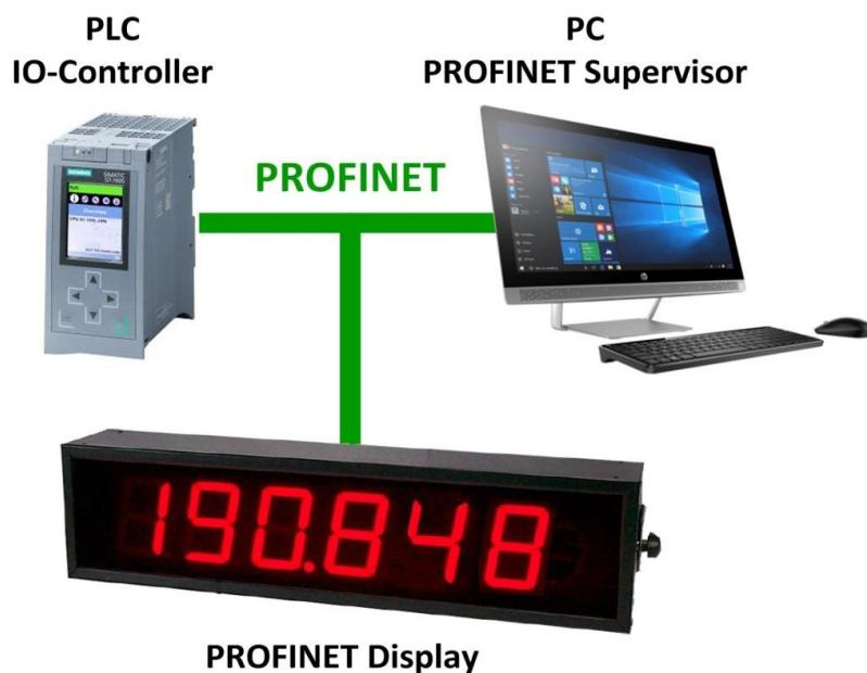
Fig. 1 Profinet communication
