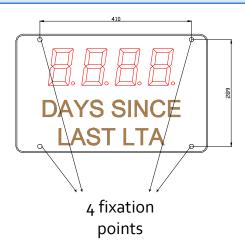
The DC-23SAC displays can be fixed to the wall in two ways:
