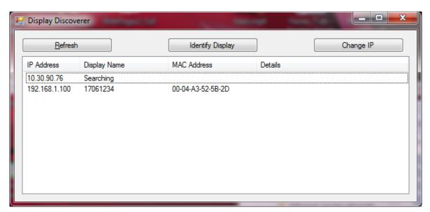
The first row shows the IP of the PC which is searching the displays and the second row a display we just have bought. As it is shown, the display has serial number 17061234 and the default IP is out of the range of the LAN. To change the IP address to a suitable one for our LAN, select the display and click the button "Change IP". When clicking this, a new window is opened where a new IP address can be tipped.
