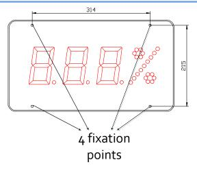
The DC-10 STHNE+2R/+4R displays can be fixed to the wall in two ways:
