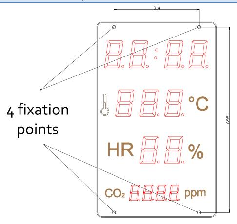
The DC-41 SRTHONE+2R/+4R displays can be fixed to the wall in two ways:
