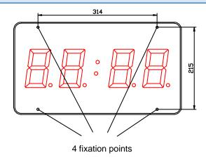
The DC-10 SR displays can be fixed to the wall in two ways:
