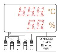
DC-25 displays are aesthetically identical to the DC-24 but do not have sensor. They must receive the data from RS-485, Ethernet or Wifi.
